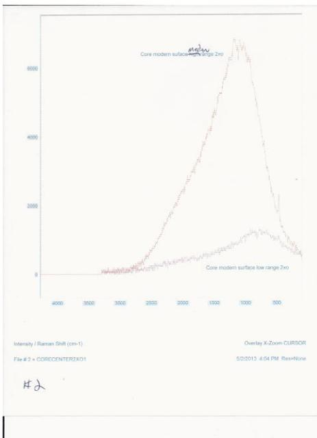
Figure 4 Raman Spectroscopy Curve Showing a Contaminated Surface
